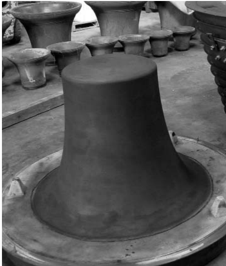
The mold for the new A3 bell ready to be closed down and cast
